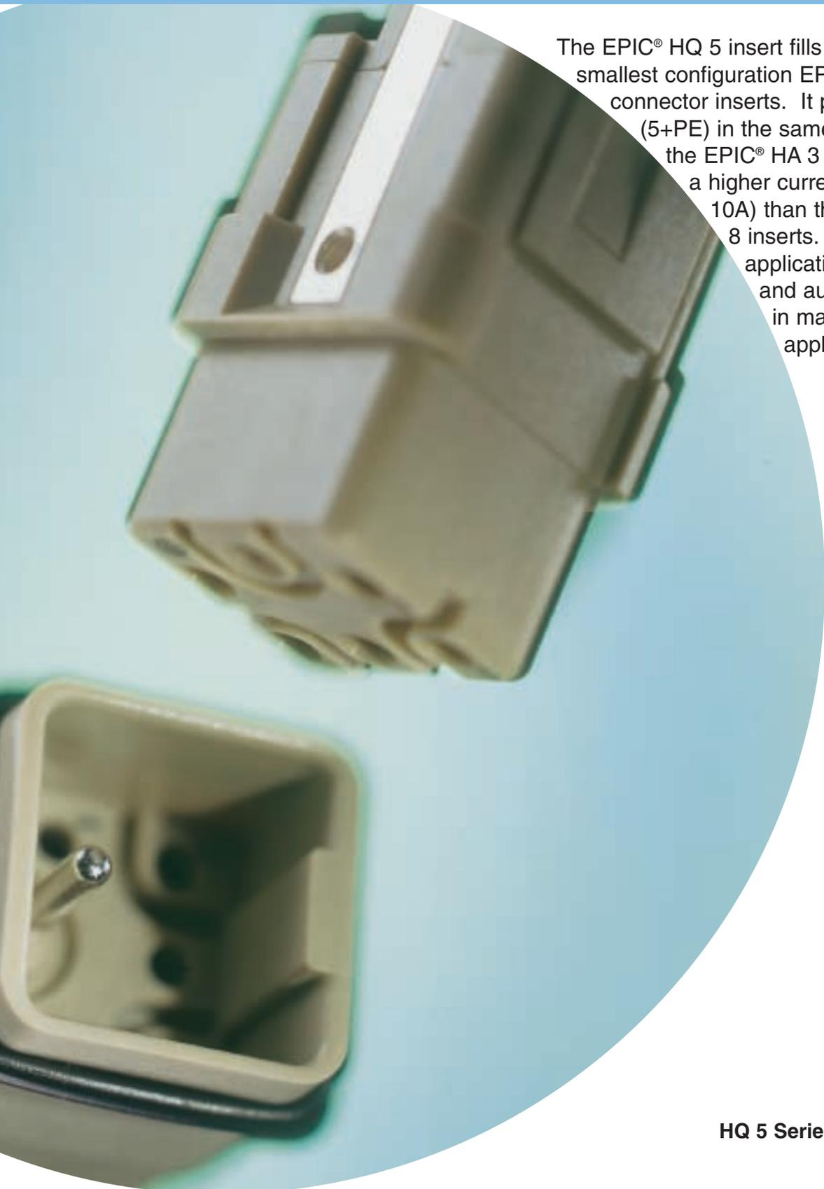
The EPIC® HQ 5 insert fills the gap between the smallest configuration EPIC® HA and EPIC® HD connector inserts. It provides more contacts (5+PE) in the same housing space as the EPIC® HA 3 and HA 4 inserts with a higher current capability (16A vs. 10A) than the EPIC® HD 7 and HD 8 inserts. They are ideal for applications in the transportation and automotive industries, and in many other industrial applications.
